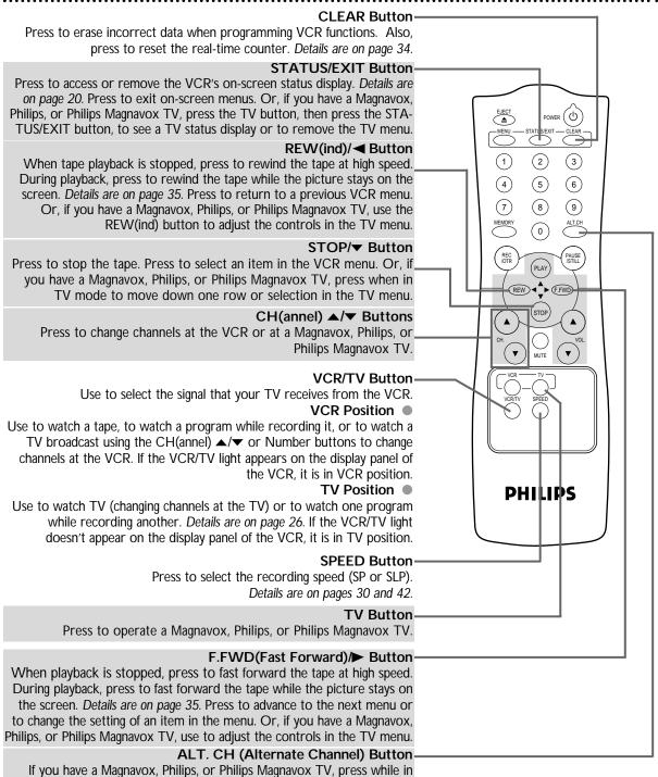
If you have a Magnavox, Philips, or Philips Magnavox TV, press while in TV position to return to the TV channel you were viewing immediately before switching to your current channel. (If you press the ALT. CH button while in VCR position, the TV will change to the channel you last selected before choosing channel 3 or 4 to use the VCR. However, the TV channel will not be clear, because you are in VCR position.)
